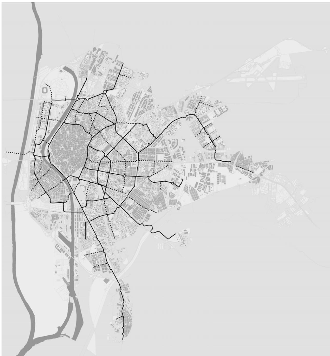
Figure 1: Evolution of the cycle network between 2006 and 2010. Solid lines show the basic network (76 km), while dashed lines show the complementary network - up to 120 km. Source: Compiled by authors from data of (Ayuntamiento de Sevilla, 2007) and (Muñoz, 2010). Further developments of the network can be found in (Ayuntamiento de Sevilla, 2013).
